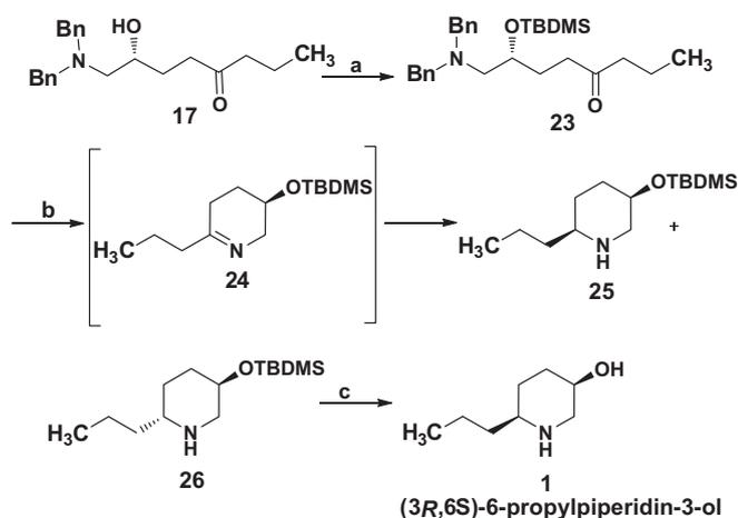
Scheme 4. (a) TBDMSCl, imidazole, DMAP, DCM (b) 10% Pd/C, EtOH (c) EtOH, IPA.HCl.
