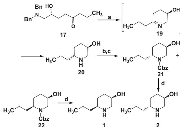
Scheme 3. (a) 10% Pd/C, EtOH, RT (b) CbzCl, Na<sub>2</sub>CO<sub>3</sub>, THF–H<sub>2</sub>O, RT (c) Separation by column chromatography (d) 10% Pd/C, EtOH.
