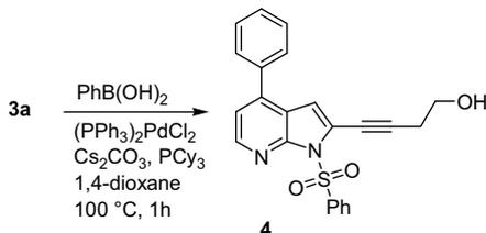
Scheme 3. Suzuki coupling of **3a** with phenyl boronic acid.
